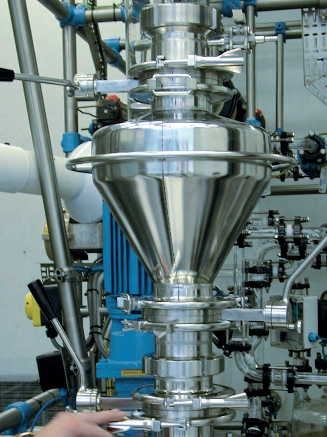
The EPTS on top of the reactor
